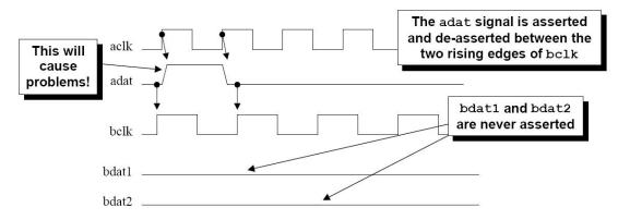
Assert the control signal for a time period longer than the slow clock period
