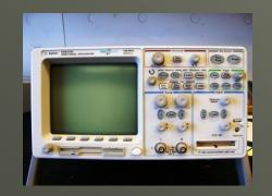
Use an oscilloscope to verify waveform generator outputs
