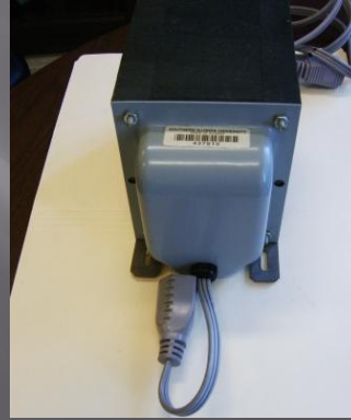
Bench-top Isolation Transformer
