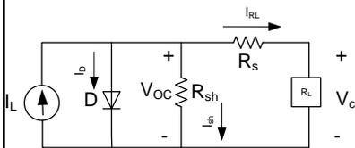
Example: Find the power delivered to a 30 ohm resistive load by the solar cell with a light current of 100 mA and model parameters of  $R_s = 1.176 \text{ } \Omega$  and  $R_{sh} = 11.875 \text{ } \Omega$ . Determine the cell load voltage for this load resistance.
