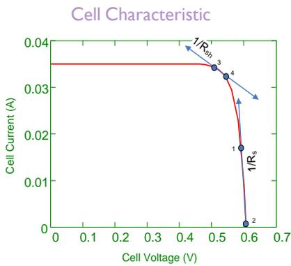
Finding Model Parameters,  $R_{sh}$  and  $R_s$
