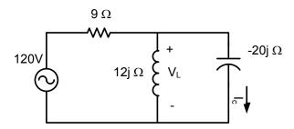
5.) The system below has a base voltage of 240V and a base power of 25 kVA find the source voltage (in actual volts) required to maintain 1 p.u. voltage on the load with the indicated current flowing.
