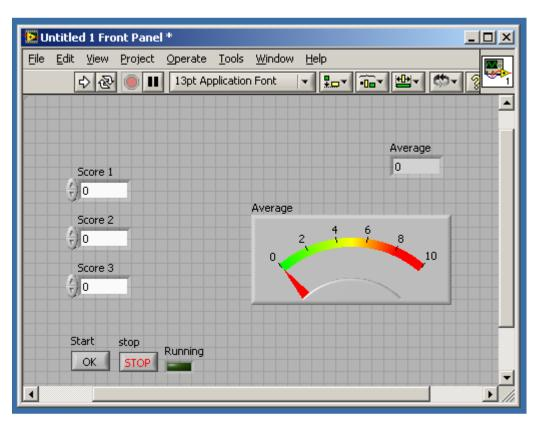
The button labeled "OK" will start an averaging operation and cause the Running LED to light. Depressing the "STOP" button ends the program. Use While loops to accomplish the desired functionality.
