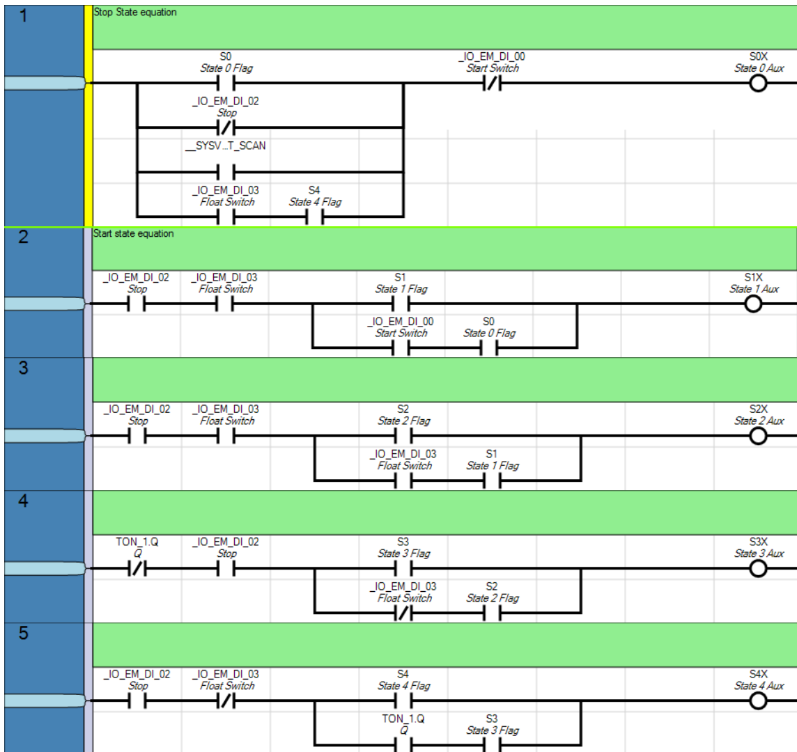
Figure 10. PLC Ladder Diagram for Example State Equations.
