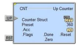
The Up Counter (CNT) has the following two ladder logic inputs:
