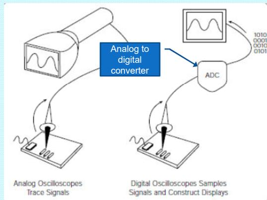
Measured voltage turned into series of samples
