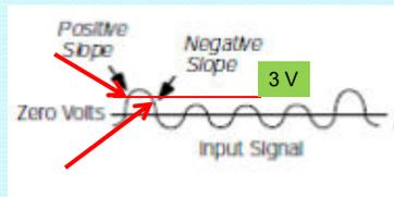
Positive Slope triggering 3V level
