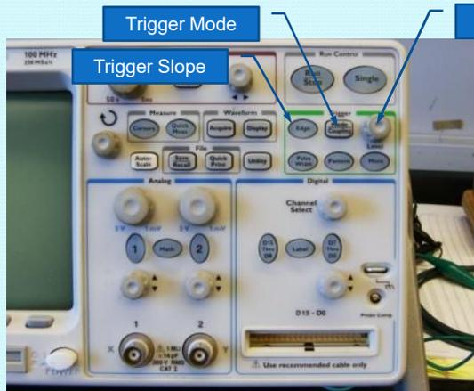
Edge and Mode buttons produce menu choices above function keys on the display
