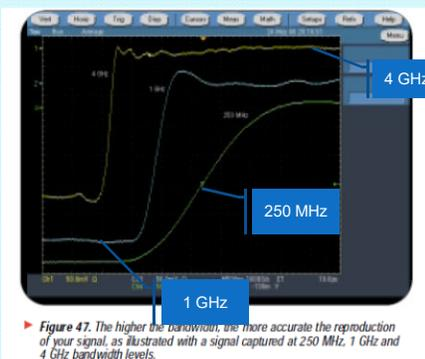
► **Figure 47.** The higher the bandwidth, the more accurate the reproduction of your signal, as illustrated with a signal captured at 250 MHz, 1 GHz and 4 GHz bandwidth levels.
