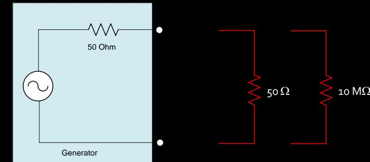
Match load to generator resistance for maximum power
