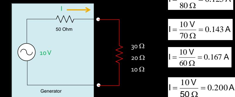
Short circuit limited by generator internal resistance
