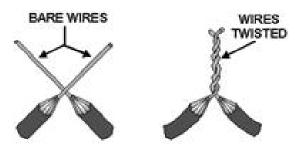
5. Strip two pieces of wire and perform the fixture splice as seen below. **On-campus students**: show the instructor your connection before continuing. **On-line students**: take a photo of the joint and import the photo into a Word document. When the lab is complete, convert the Word document to a pdf and submit it with your lab documentation to the assignment in the course.
