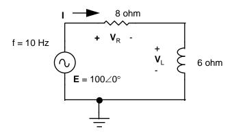
Convert the phasor source voltage E to a peak value with the appropriate phase shift for use in the simulator.
