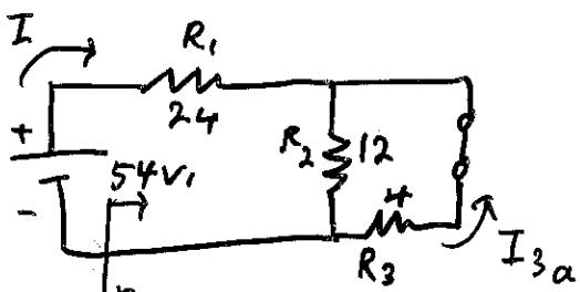
$$R_T = R_1 + R_2 // R_3$$
