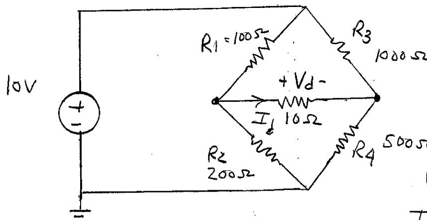
$$\frac{R_1}{R_2} = \frac{100\Omega}{200\Omega} = \frac{1}{2}$$
