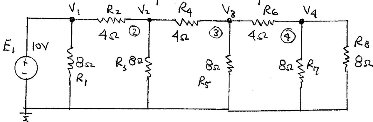
Voltage known at  $V_1$   $V_1 = E_1$
