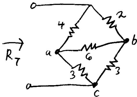
In order to simplify the network we can replace the  $\Delta$  section with a  $\Upsilon$  section
