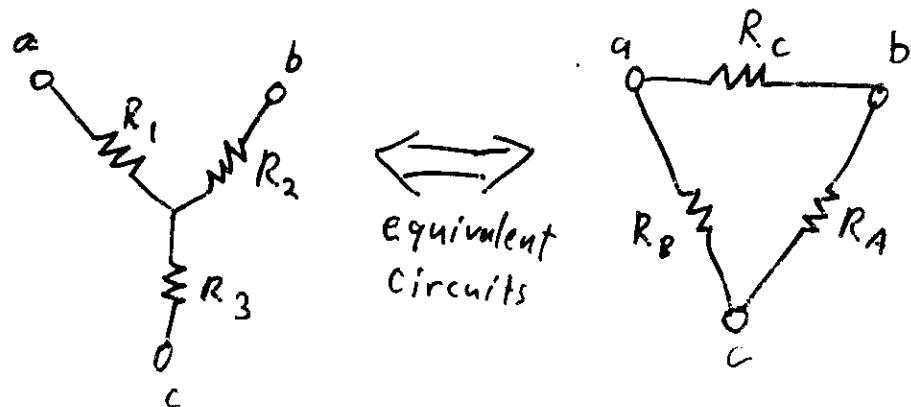
$$\underline{\Delta \rightarrow Y \text{ Conversion}} : R_1 = \frac{R_B R_C}{R_A + R_B + R_C} \quad R_2 = \frac{R_A R_C}{R_A + R_B + R_C} \quad R_3 = \frac{R_A R_B}{R_A + R_B + R_C}$$
