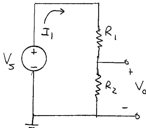
$$V_o = \frac{R_2}{R_1 + R_2} V_s$$
