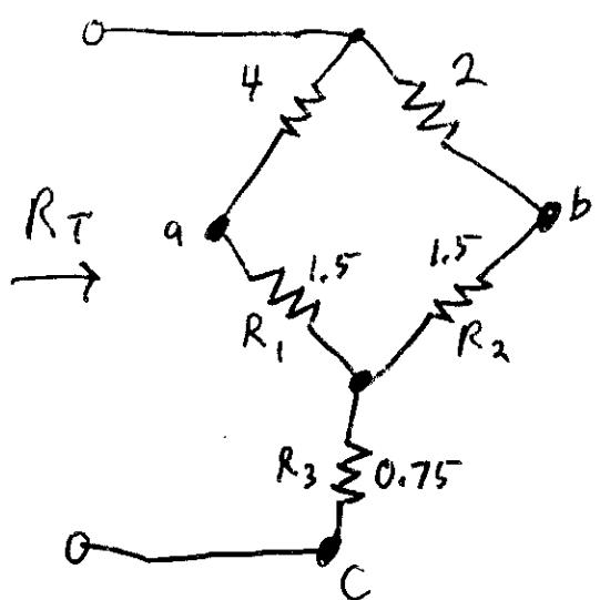
In this new equivalent ckt. it is possible to use series and parallel resistor combining rules to simplify the network.
