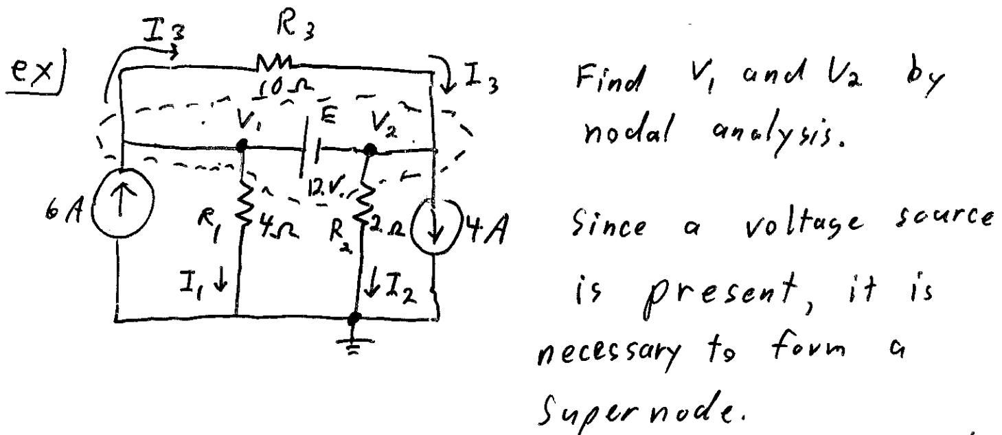
(Note: all of the currents crossing the boundary of the supernode can be found with  $\text{KCL}$  or are given)
