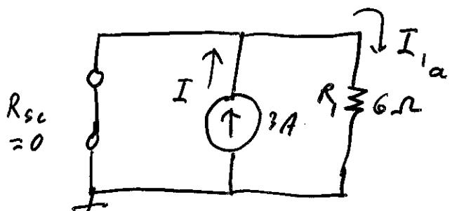
(Note:  $I_{1a}$  is the part of  $I_1$  due to the 3A. Source)
