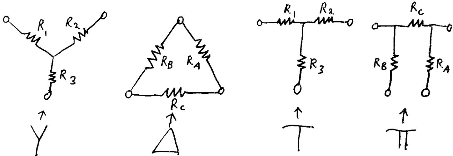
The  $Y$  and the  $T$  are identical circuits that are drawn differently.
