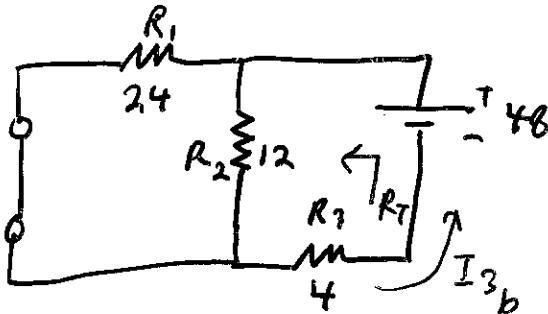
$$R_T = R_3 + R_1 // R_2$$
