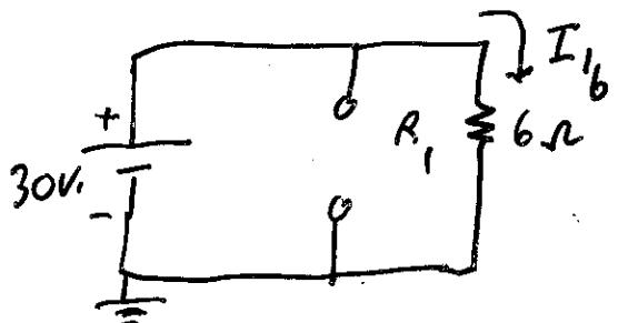
(Note:  $I_{1b}$  is the part of  $I_1$  due to 30V. source)
