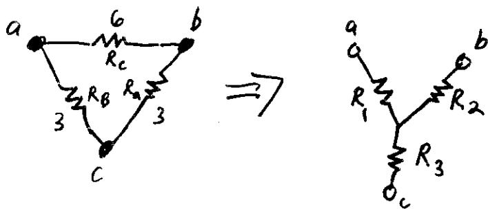
Using the conversion formulas to find  $R_1, R_2, R_3$  gives:
