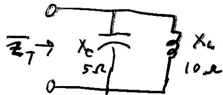
$$\bar{Z}_T = \frac{\bar{Z}_C \bar{Z}_L}{\bar{Z}_C + \bar{Z}_L}$$
