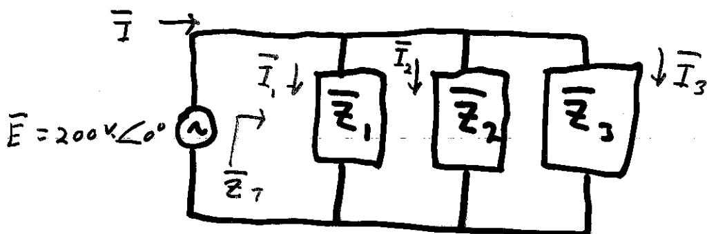
$$\bar{Z}_1 = R_1 = 10 \angle 0^\circ \Omega$$
