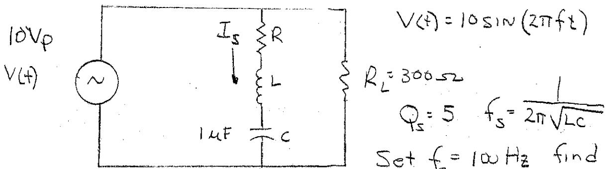
$$\frac{1}{2\pi f_s} = \sqrt{LC} \quad \left(\frac{1}{2\pi f_s}\right)^2 = LC \quad \left(\frac{1}{2\pi f_s}\right)^2 \frac{1}{C} = L \quad L \text{ (Henry)}$$
