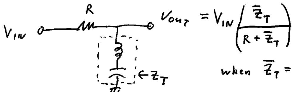
$$V_{out} = V_{in} \left( \frac{\bar{Z}_T}{R + \bar{Z}_T} \right)$$
