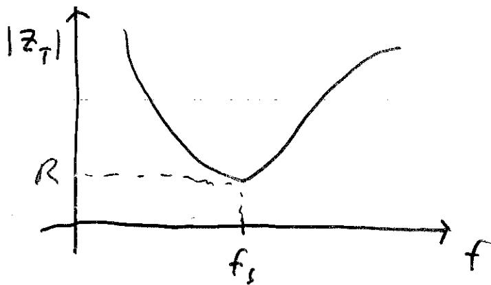
$|Z_T|$  is a minimum at resonance for the series RLC circuit
