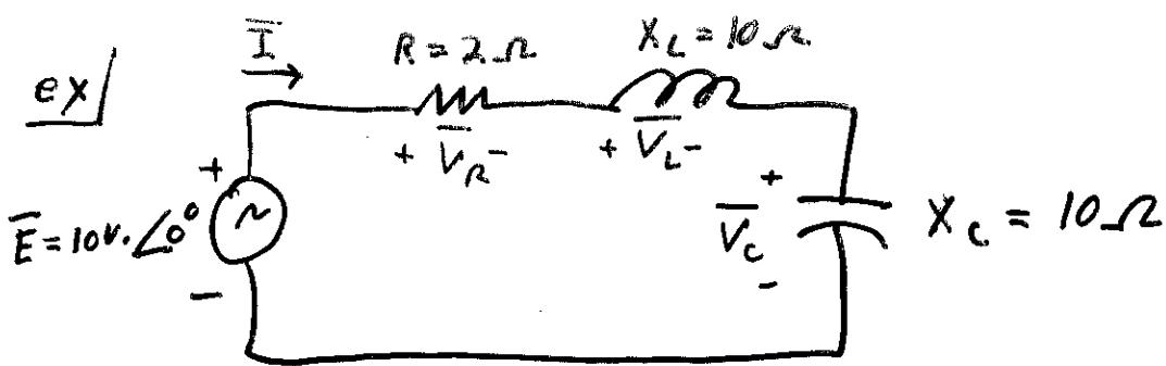
a) Find  $\bar{I}$ ,  $\bar{V}_R$ ,  $\bar{V}_L$  and  $\bar{V}_C$  for series resonant ckt.
