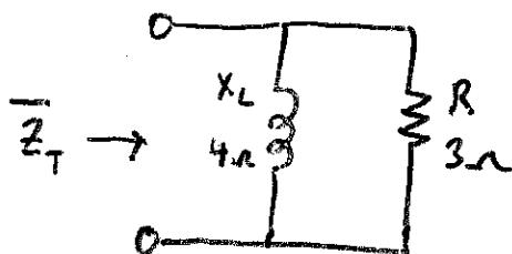
$$\bar{Z}_T = \frac{\bar{Z}_L \bar{Z}_R}{\bar{Z}_L + \bar{Z}_R} = \frac{(4 \angle 90^\circ)(3 \angle 0^\circ)}{4 \angle 90^\circ + 3 \angle 0^\circ}$$
