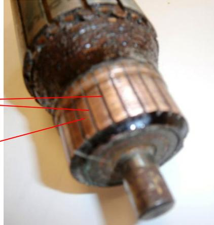
Segments connect the armature coils to the load through the brushes.
