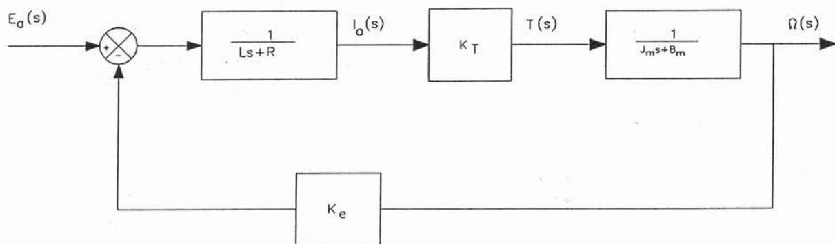
Note that the dc motor has an inherent feedback from the cemf
