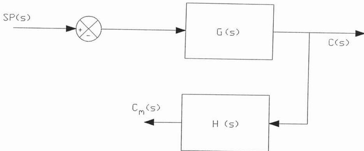
In the open loop mode the error signal is equal to the setpoint value.
