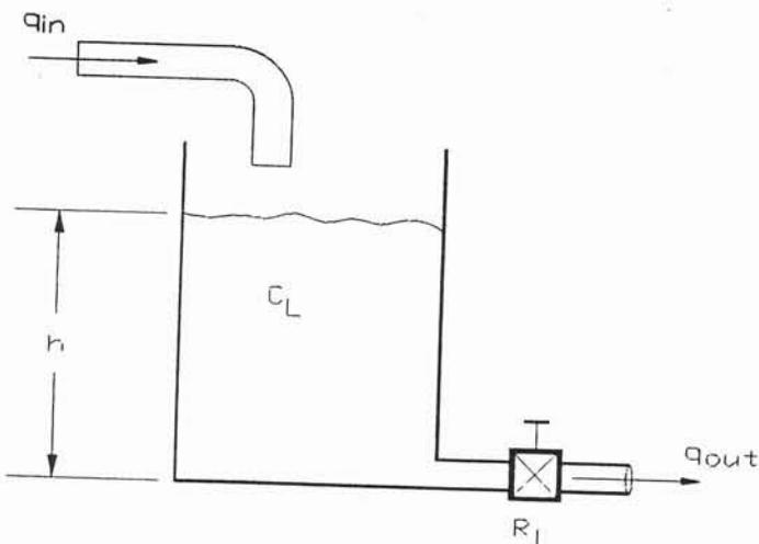
Process input:  $q_{in}$  = input flow rate (% FS<sub>in</sub>)
