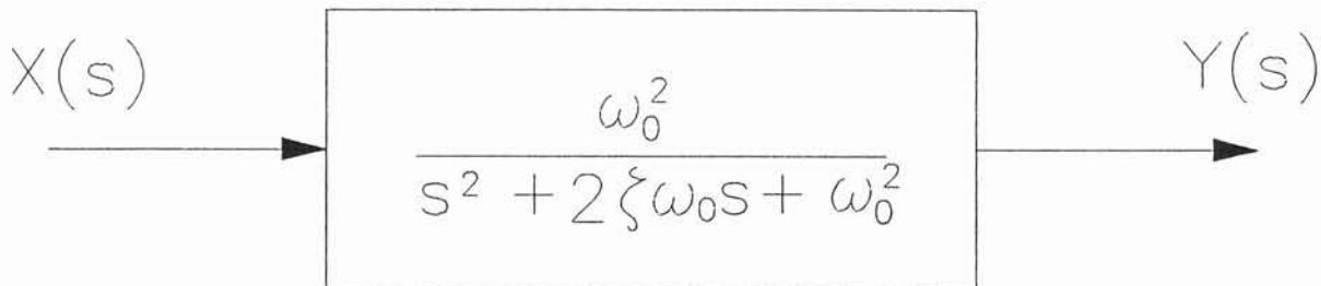
Transfer Function using standard notation for a second order system
