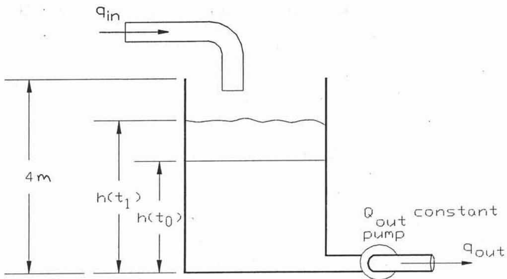
For tank system shown, find the transfer function when tank diameter = 1.5 m and h = 4 m. Full scale
