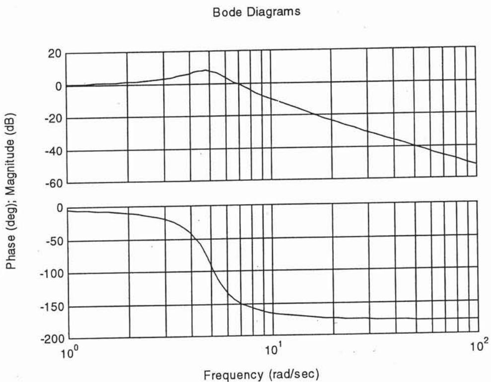
This shows a resonant peak at the resonant frequency
