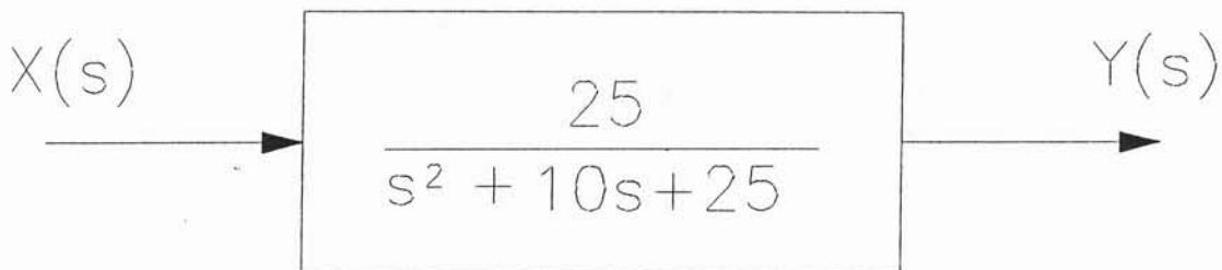
Find  $\omega_0$  and  $\zeta$  for this system and determine if the system is critically, under or over damped
