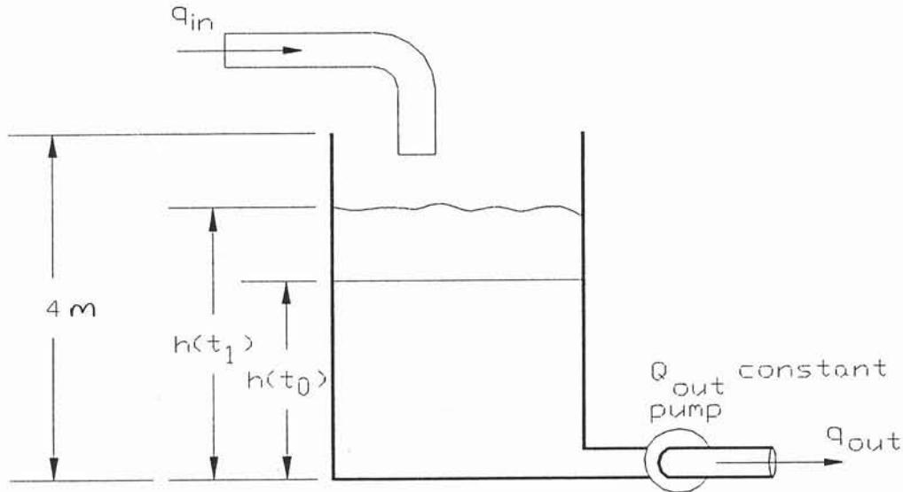
$$h(t) - h(t_0) = \frac{1}{T_i} \int_{t_0}^{t_1} (q_{in} - q_{out}) dt \quad t_1 = 100 \text{ s} \quad h(t_0) = 22.5\% (0.9 \text{ m})$$
