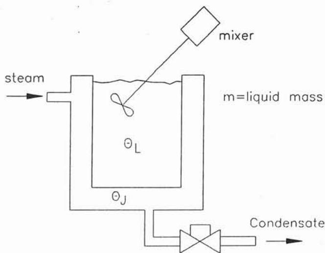
Temperature of oil bath  $\theta_L$  depends on the steam temperature  $\theta_J$  and the thermal resistance and capacitance of the system
