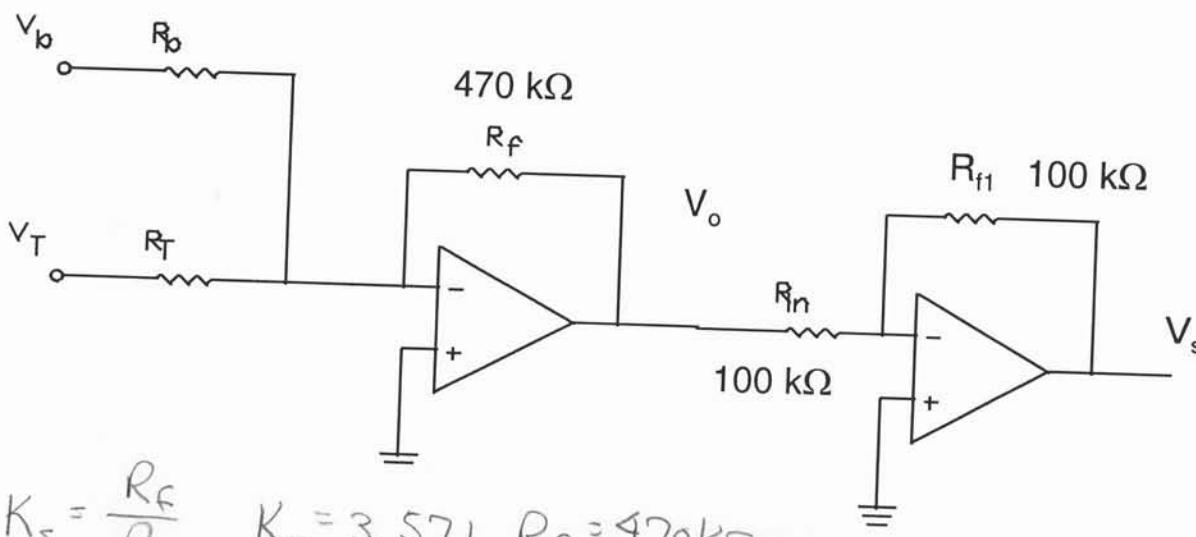
$$K_s = \frac{R_f}{R_T} \quad K_s = 3.571 \quad R_f = 470 \text{ k}\Omega$$
