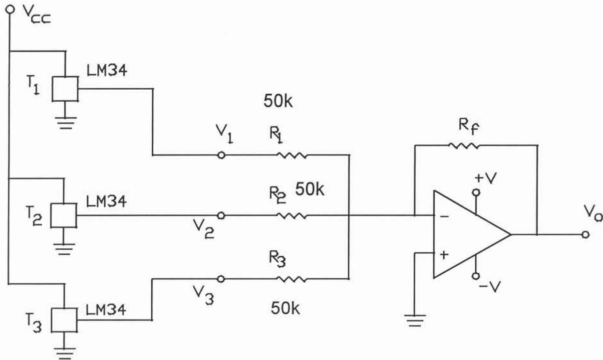
LM34 - temperature sensors. Gain = 10 mV/F
