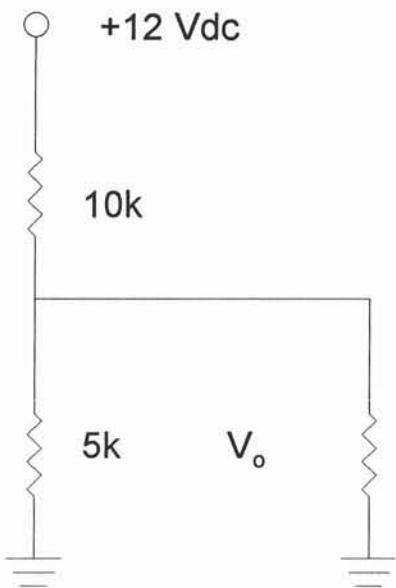
Voltage divider formula only valid for infinite load resistance
