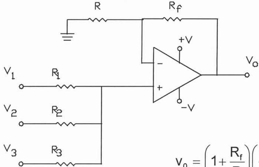
$$V_o = \left(1 + \frac{R_f}{R}\right) \left(\frac{V_1 + V_2 + V_3}{3}\right)$$
