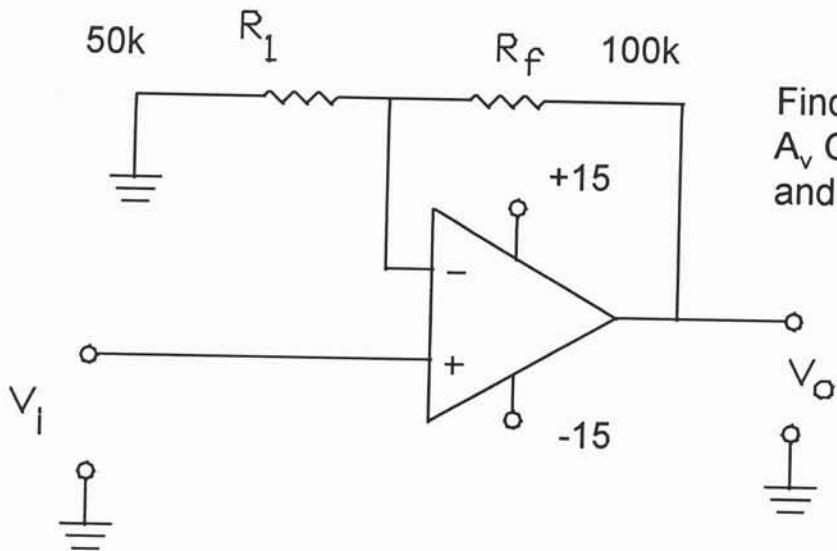
Find  $V_o$  and  $A_v$  Given values of R and  $V_i = -1 \text{ Vdc}$
