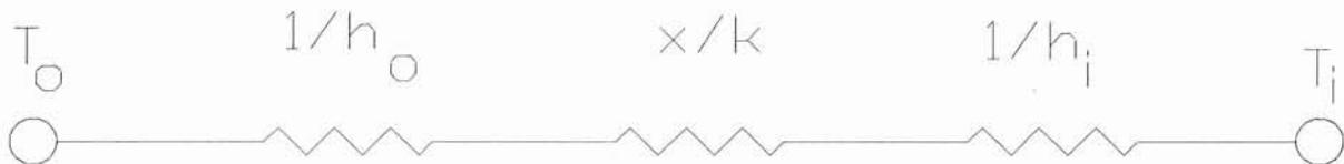
$$R_u = \frac{1}{h_o} + \frac{x_1}{k_1} + \frac{x_2}{k_2} + \dots + \frac{x_n}{k_n} + \frac{1}{h_i} \quad \text{K-m}^2/\text{W}$$
