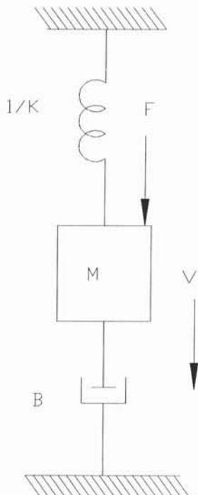
Mechanical Capacitance - change in length of spring required to make unit increase in force. Inverse spring constant
