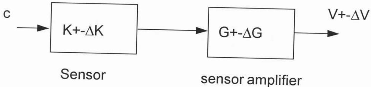
$K$  = sensor gain     $G$  = amplifier gain
