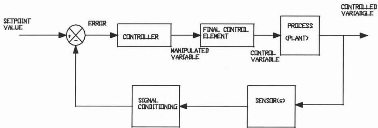
Simplest form of controller - amplify error and apply signal to the process through final control element.
