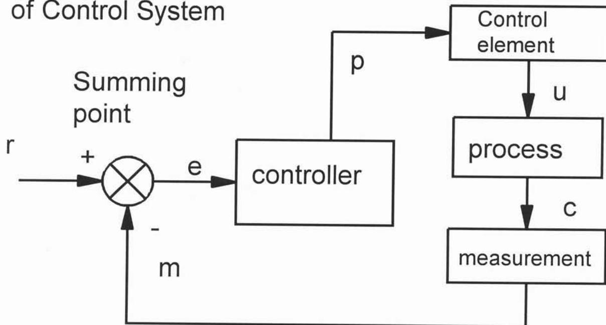
Signals form a loop   Control loop
