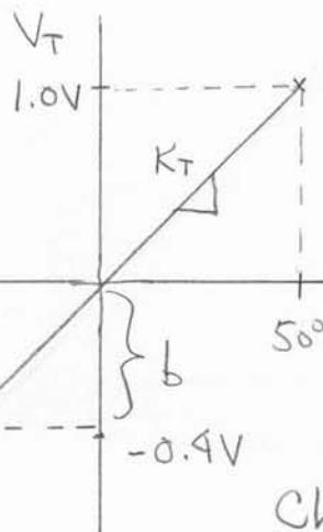
$$K_S = \frac{S_d}{S_T} = \frac{(5-0)\text{V}}{1-(-0.4)} = 3.571 \text{ V/V}$$
