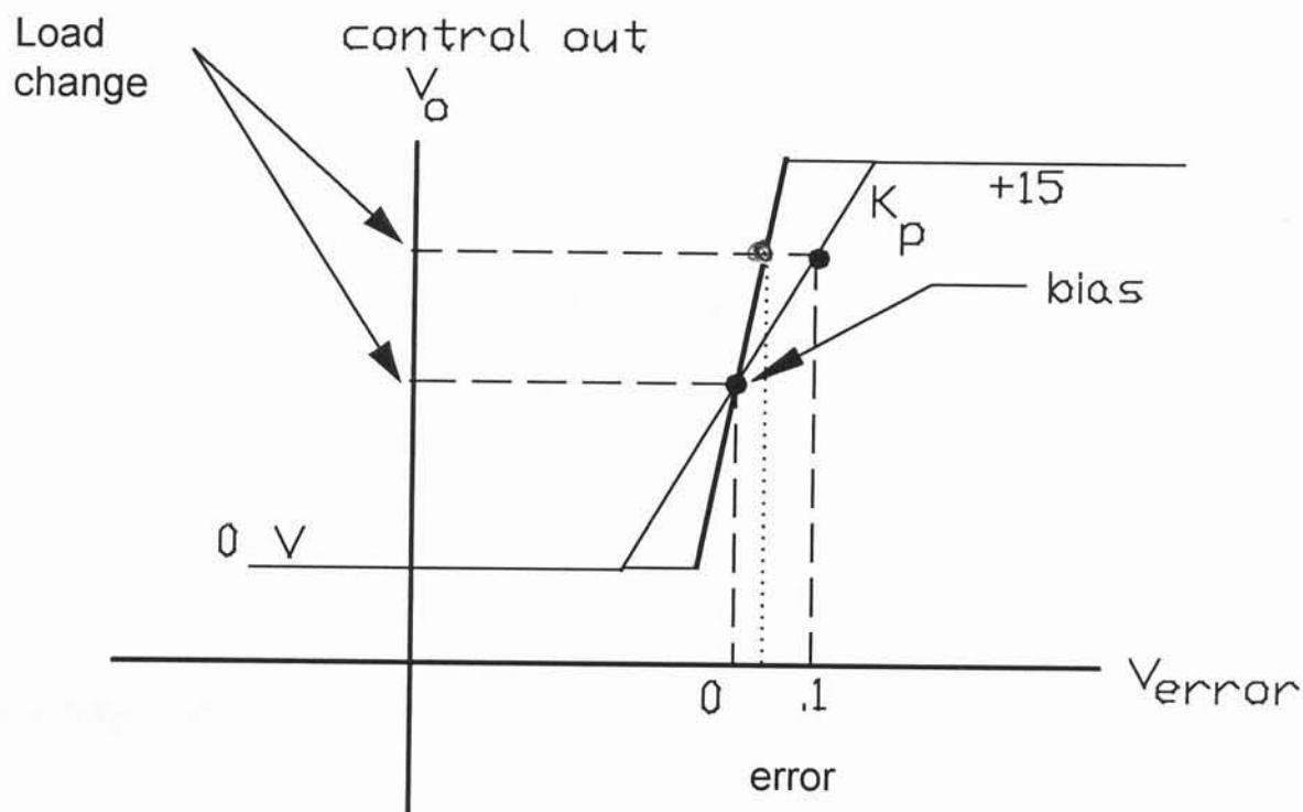
If the load change is permanent, then the error is permanent. Increasing  $K_p$  decreases steady-state error but can not eliminate it.
