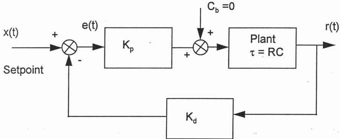
$K_d$  = feedback gain (voltage divider in lab)
