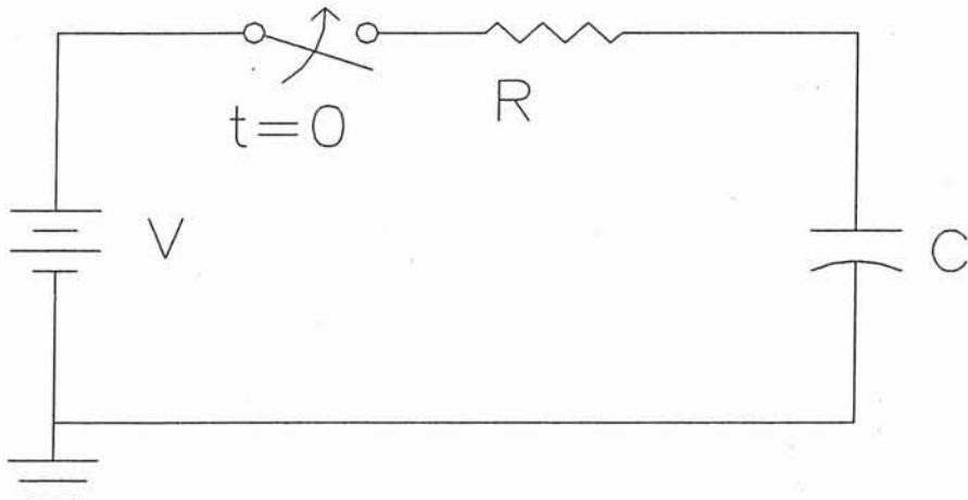
1.) Write integro-differential equation Using KVL
