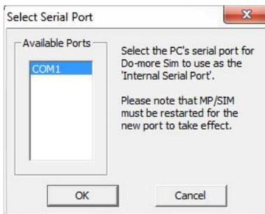
The Do-more Simulator can use one of the computer's onboard serial ports as the Internal Serial Port (@IntSerial). The **Sim-> Select Comm Port** menu selection will open this dialog which will list the available serial ports on the computer. Highlight the serial port in the list to use and click OK.
