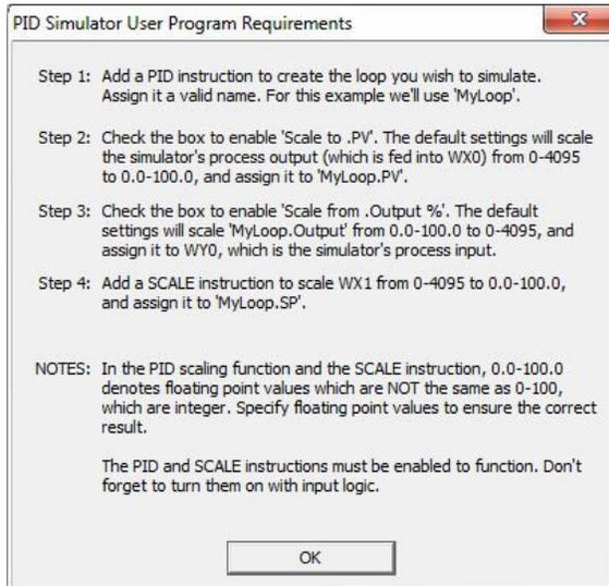
Add a [Closed Loop Controller \(PID\)](#) instruction with the following parameters:
